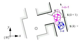
Here the robot pose has been predicted based on odometric information
