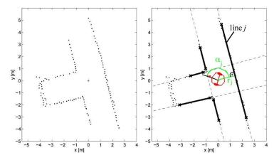
From laser data line features are extracted using a least square fit
