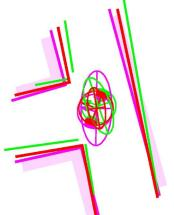
The predicted model (purple) and the measured data (green) are combined in the Kalman update step to refine the estimate (red) and the process can be repeated.
