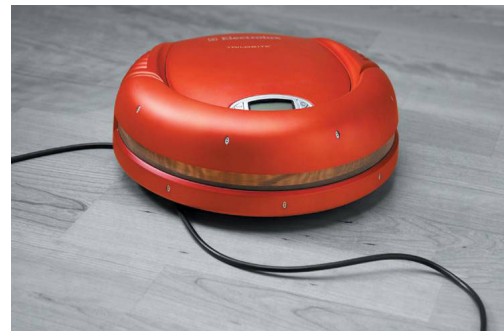
Figure 6: The Electrolux Trilobite vacuum cleaner, for domestic use, that is commercially available.
