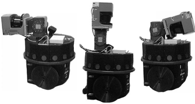
Figure 1: The SuperScout Louie with a PTU mounted SICK.
