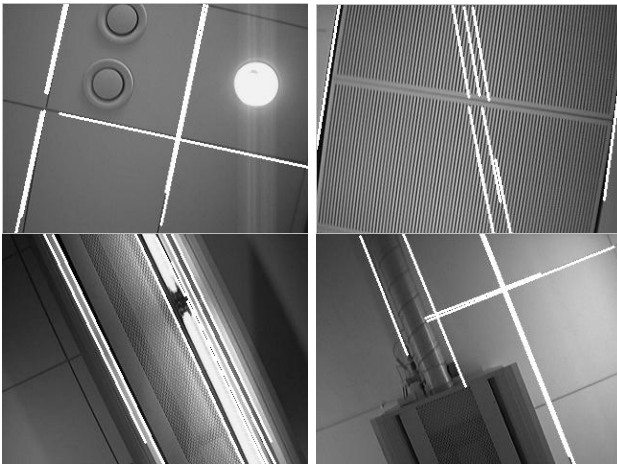
Fig. 3. Snapshots of the ceiling along the path showing the line detection output.
